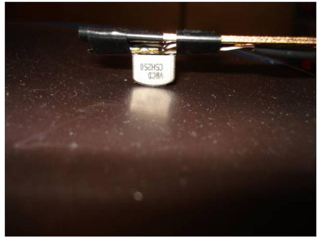
Figure 3: Close-up of the magnetic tape head.
