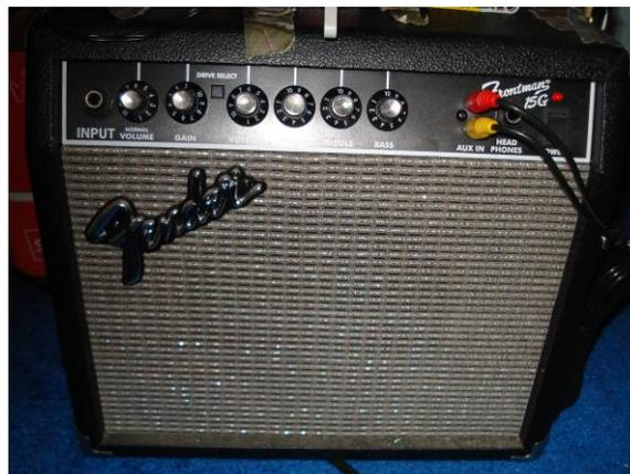
Figure 4: The amplifier. Note that the yellow and red coaxial cables lead directly from the tape head into the amp.
