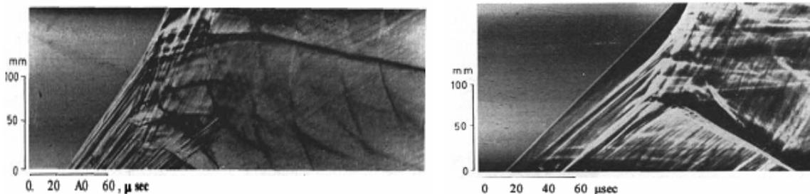
Figure 2. Soloukhin's Schlieren streak images of detonation formation in mixture of natural gas and oxygen (left) and in hydrogen-air mixture (1958).
