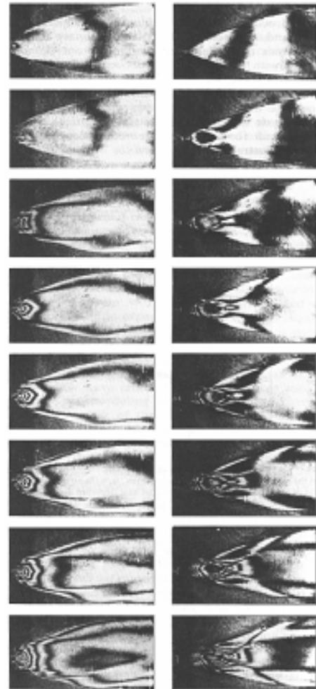
Michelson interferometer frame records of starting processes in mixing gasdynamic lasers [17]. Time interval between frames is varied up to 1 μs.
