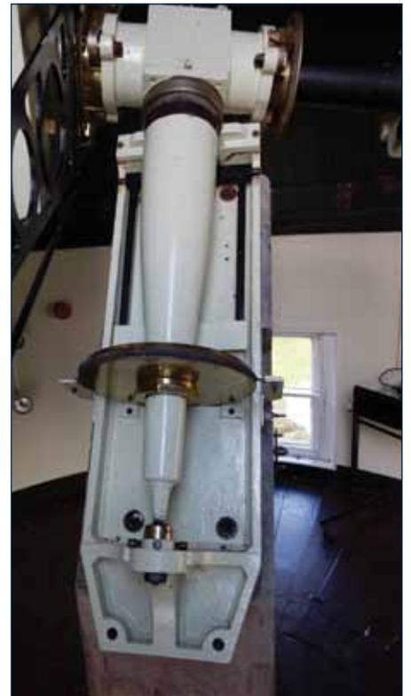
Fig. 5 The cradle holding the polar axis mounted on the south side of the stone pier. Note the now redundant circular brass gearwheel which it is believed may have been meshed with the driving clock in the original configuration.
