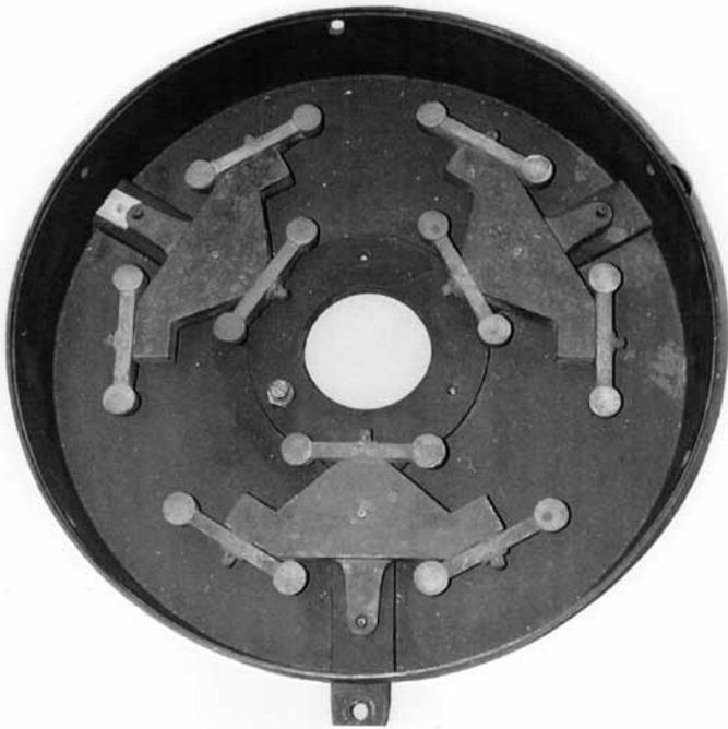
Fig. 4 The 9-lever, 18-point, mirror support cell for the 15-inch telescope.
