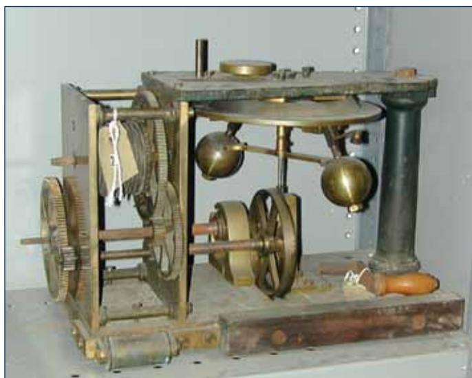
Fig. 7 An almost identical driving clock by Grubb at Dunsink Observatory to that for the Armagh 15-inch telescope. This version has its original governor. The short worm-wheel is behind and to the left of the gear connecting to the governor.
