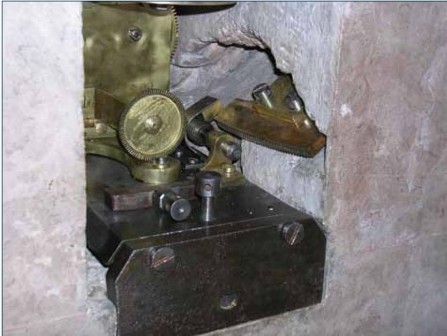
Fig. 6 The driving clock for the 15-inch telescope, minus its governor, in its second, final, position in the middle of the stone pier. Note the sector, appearing in the cutaway stone to the right and the short worm-wheel immediately to its left attached to the clock drive.
