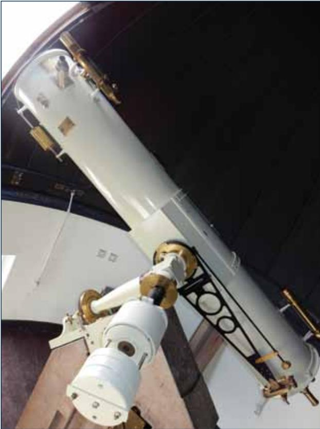
Fig. 9 The restored Grubb 15-inch reflector in the 1827 dome at Armagh Observatory.
