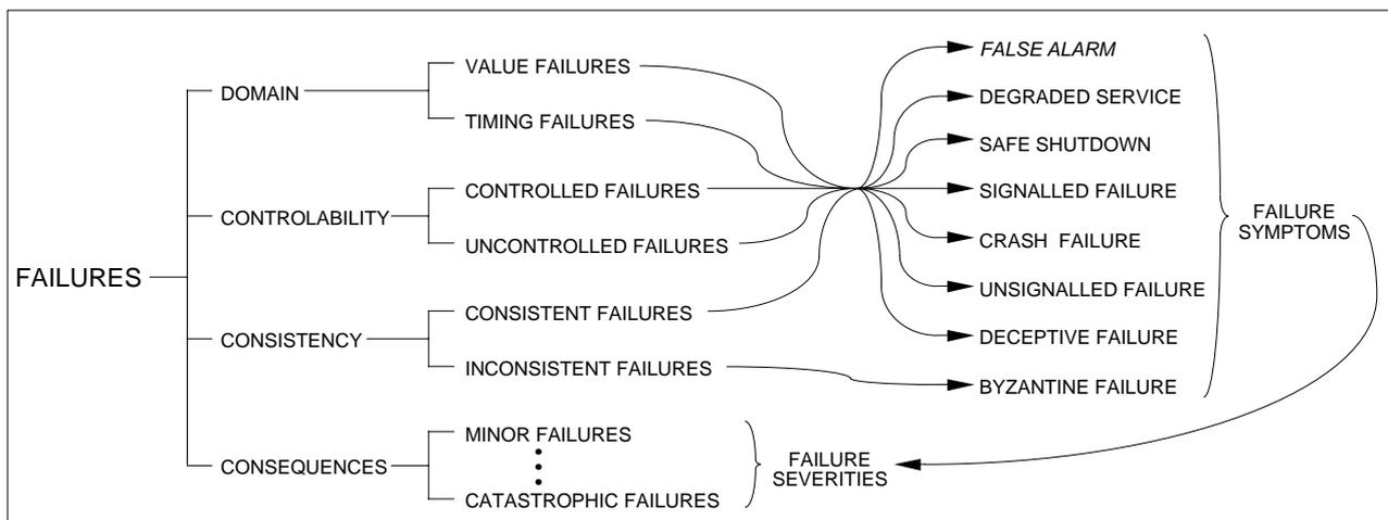
Figure 2 - The failure modes
