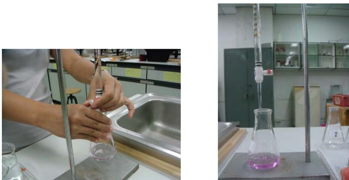
**Figure 4.** In standard buret titration, around 10-40 cm<sup>3</sup> of chemicals was used.
