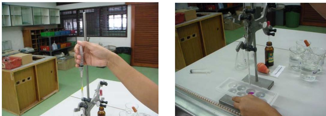
**Figure 3.** In microburet module titration, only 5-25 drops of chemicals were used.
