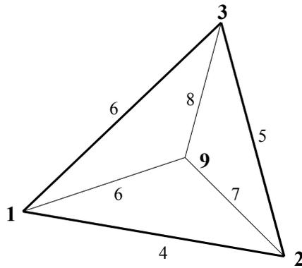
*Figure 7. The HCT Compatible Plate Bending Element*
