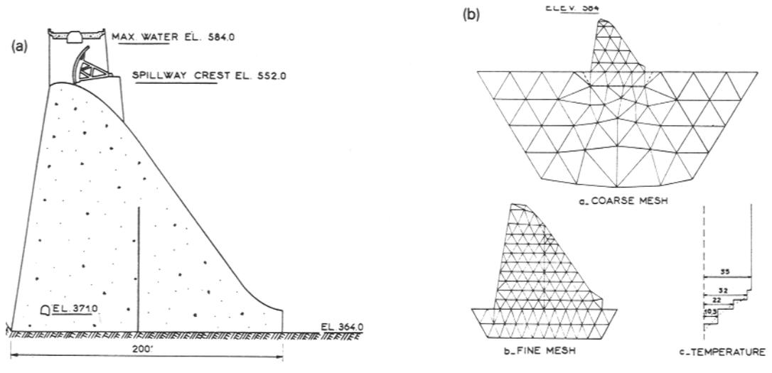
**Figure 4. The Finite Element Analysis of Norfolk Dam**
