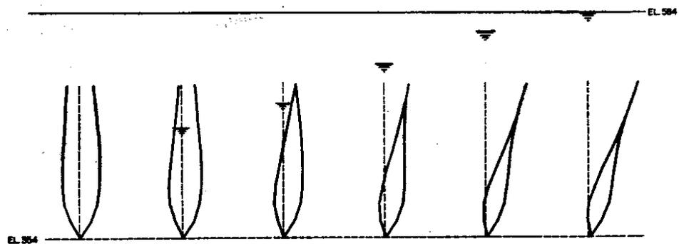
**Figure 5. Crack Closing as Reservoir is Filled**
