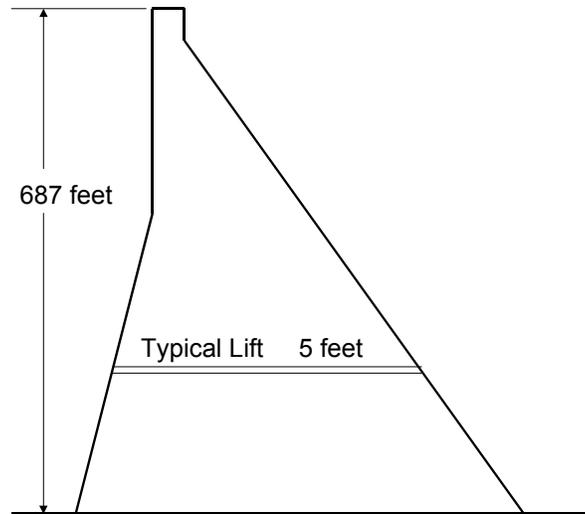
***Figure 8. Evaluation of Construction and Creep Stresses in Dworshak Dam***
