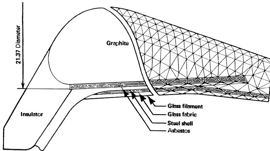
*Figure 10. Finite Element Analysis of Rocket Nozzle*
