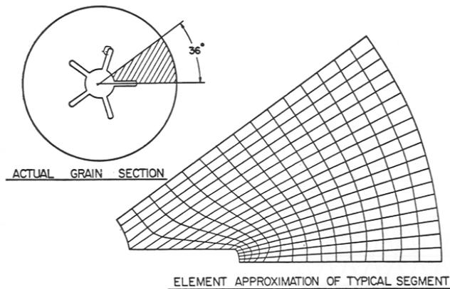
**Figure 9. Finite Element Analysis of Solid Rocket Motor**
