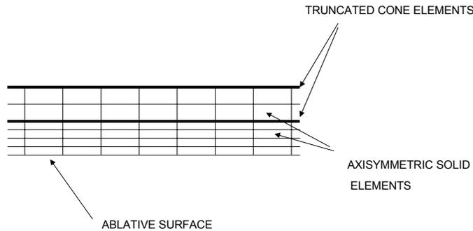
*b. Finite Element Model of Heat Shield*
